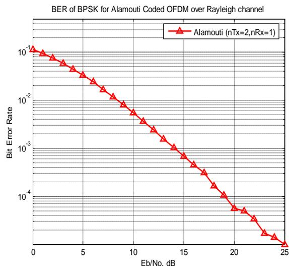
Figure 6 : Simulated BER Vs SNR of OFDM with Alamouti STBC (MISO-OFDM)
